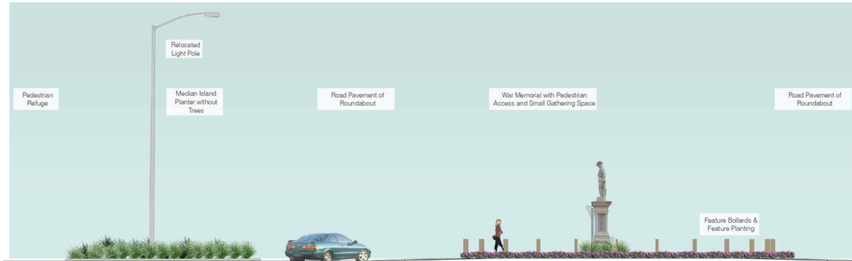
LANDSCAPE SECTION B - THROUGH ROUNDABOUT scale 1:100@A3
