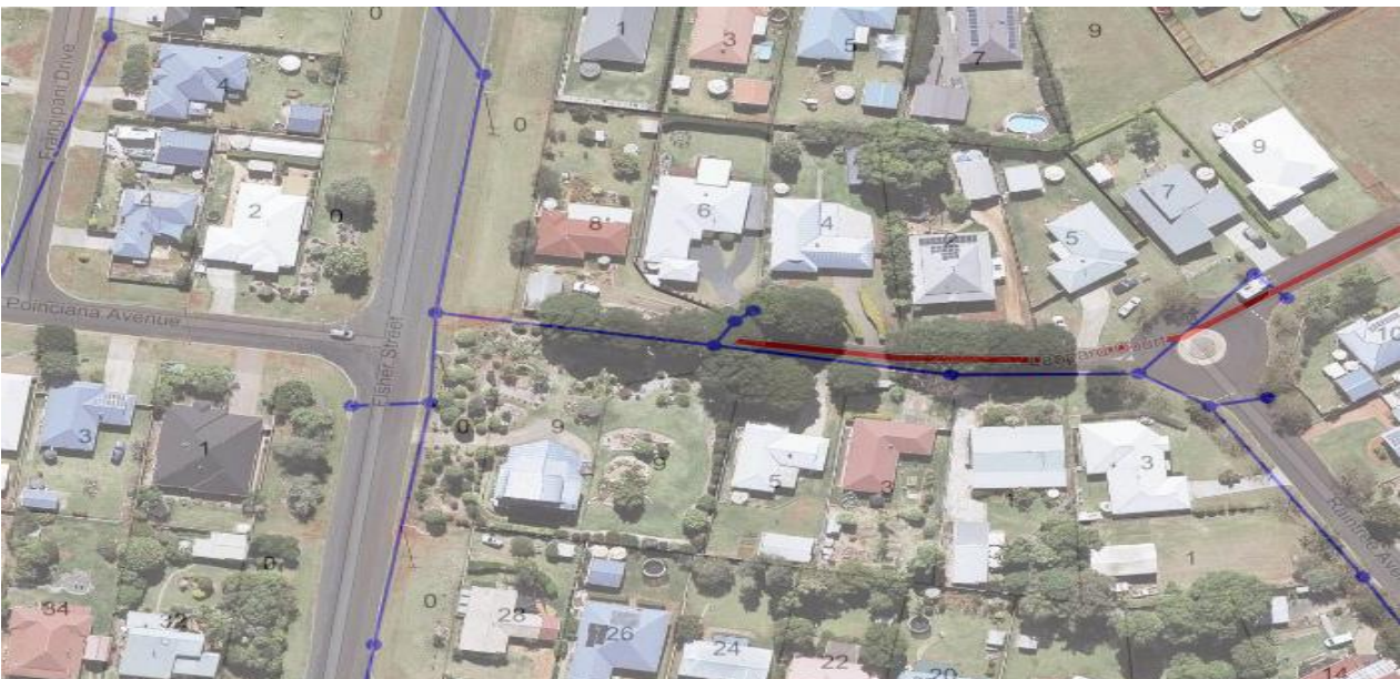
Existing underground stormwater pipe network runs along the easement
