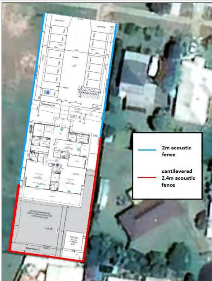
Figure 1 – Acoustic barrier specifications.
