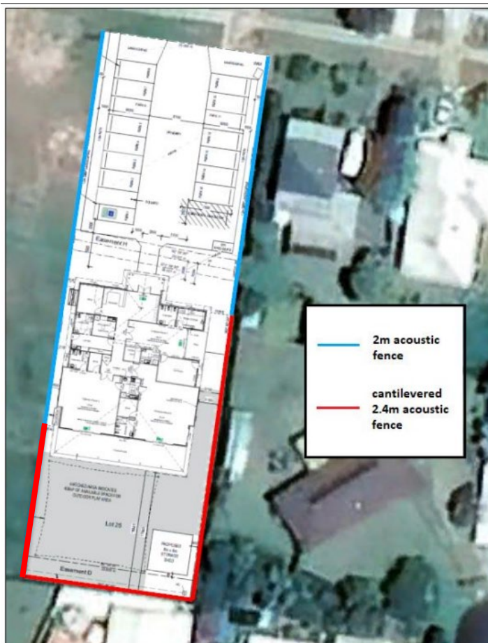
Figure 1 – Acoustic barrier specifications.
