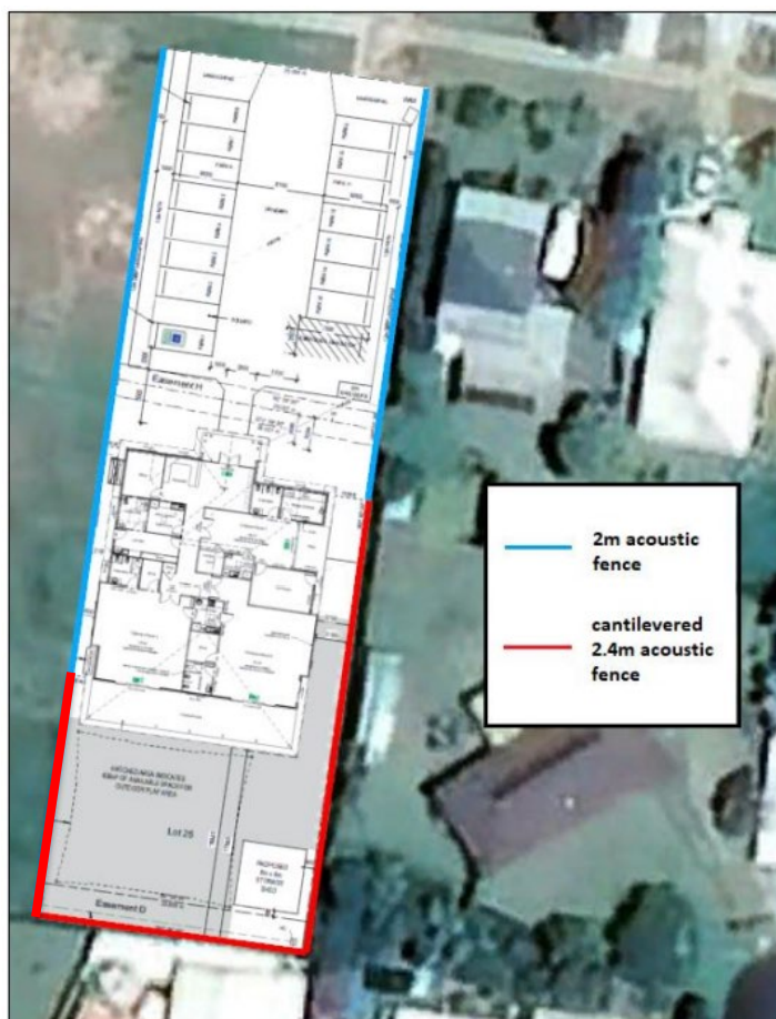
Figure 1 – Acoustic barrier specifications.
