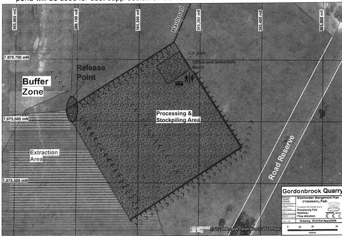
Figure 9 – Processing & Stockpiling Area Stormwater Management Plan (source: NV Engineers (QLD) Pty Ltd, 2022)
