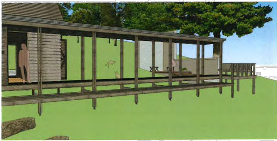
Figure 02: Front verandah and decorative timber bench seat showing twin post detail
