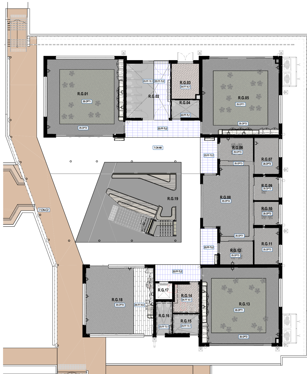
1 DA - GROUND LEVEL - FLOOR FINISHES PLAN 1:100
