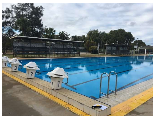
50m Pool with wet edge side walls and end headwalls with starting blocks at deep end.
