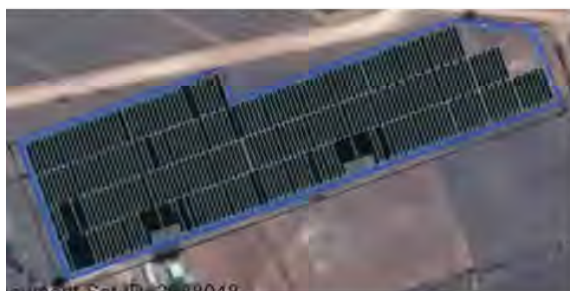
6MWp PEG aligned to the site boundaries
