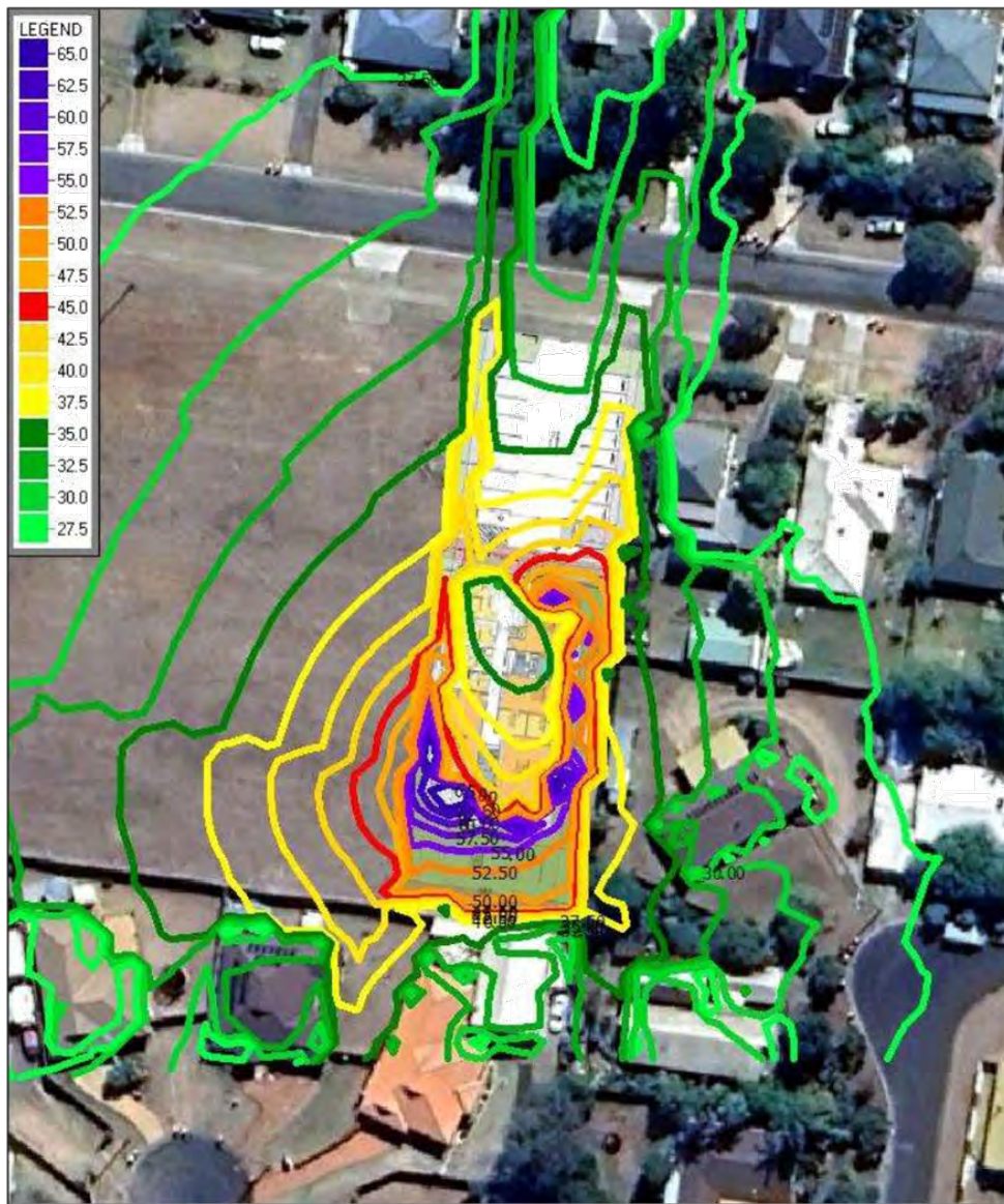
Noise contours at 1.8m, breakout from indoor play. Levels are in dB(A) L_{eq,1hr}
