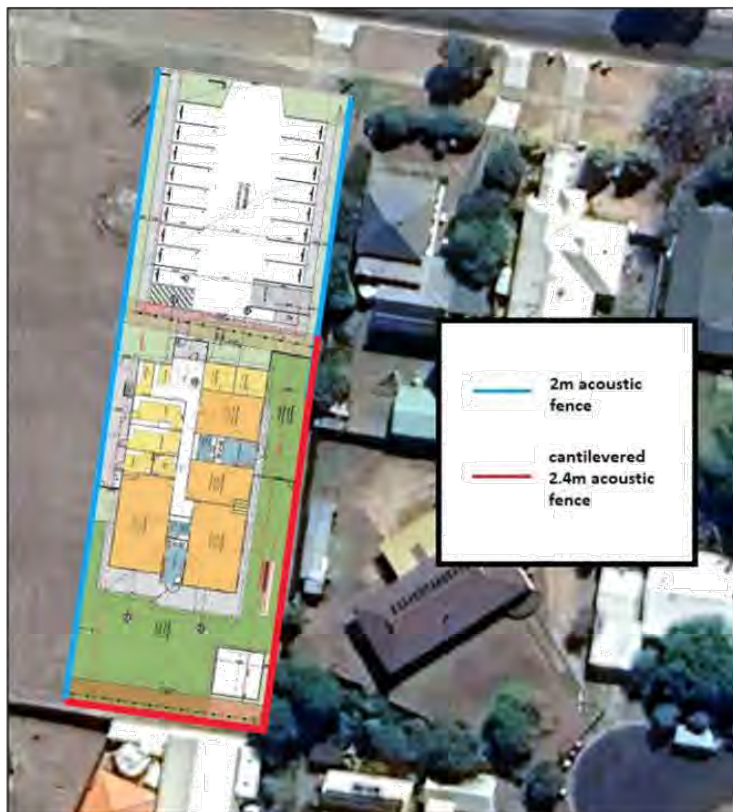
Amended Figure 1 Recommended acoustic barrier specifications
