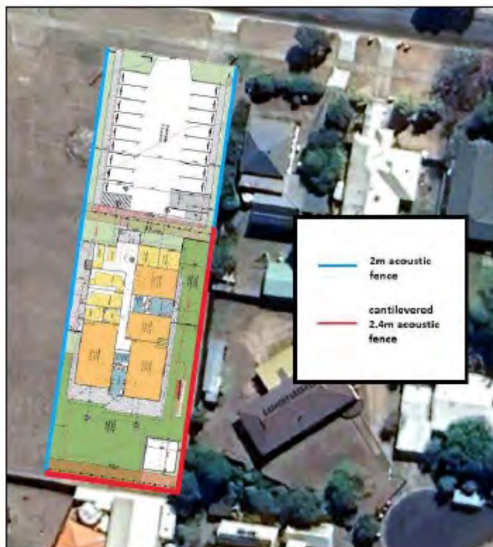
Amended Figure 1 – Recommended acoustic barrier specifications.
