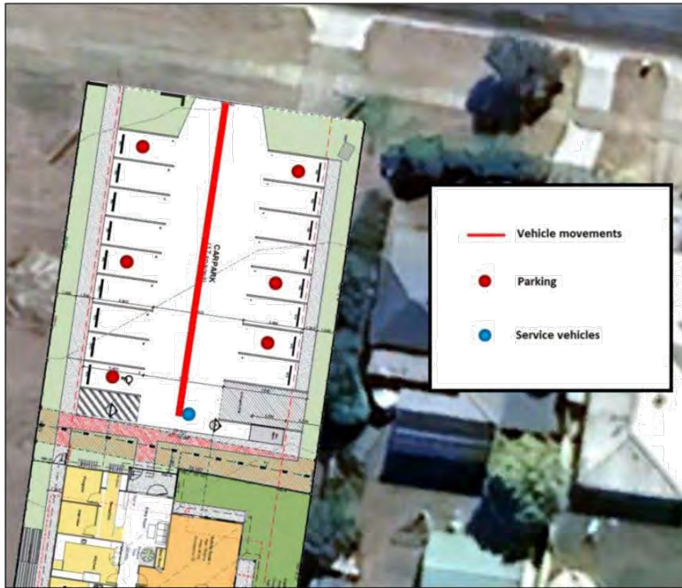
Noise source locations, carpark
