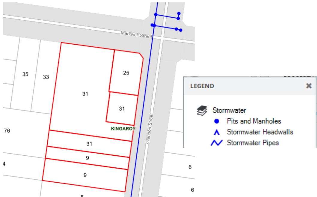
Figure 6 - Source: IntraMaps (Stormwater Network).
