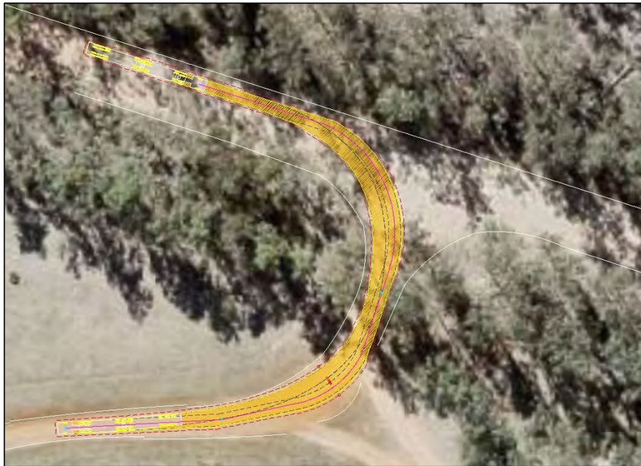
Figure 6-6: Swept path assessment (26m B-Double) – Right into Site Access from Memerambi Barkers Creek Road
