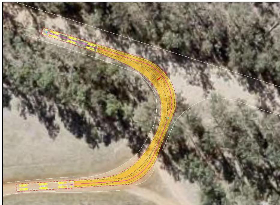
Figure 6-7: Swept path assessment (26m B-Double) – Left out of Site Access onto Memerambi Barkers Creek Road
