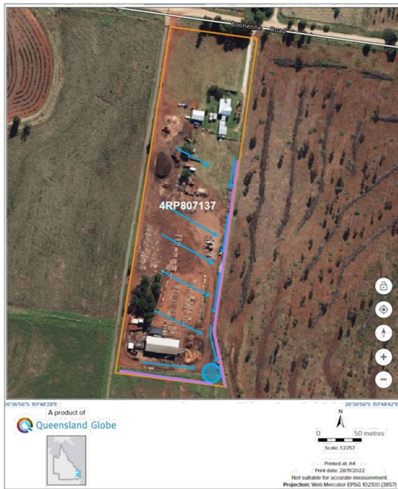
Diagram 5: Indicative stormwater flow paths on the site (purple line on east and south boundaries depicts earth / chip bund, blue circle represents a sediment basin (base figure Qld Globe, November 2022)).
