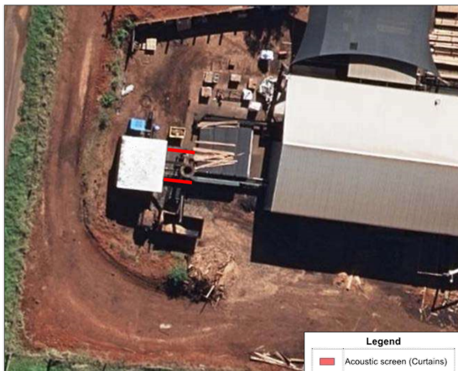
Figure 5.1 Alignment of acoustic screen (shredder shed)
