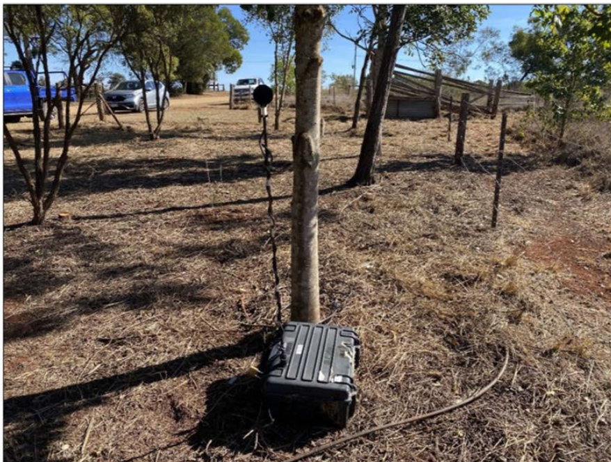
Photo 2: Noise measurement (Front-end loader) – view due west
